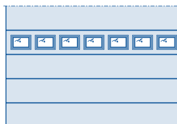
Version with panel glazing type S Glazing dimensions (W × H): 395 × 270 Clear view (W × H): 327 × 202
